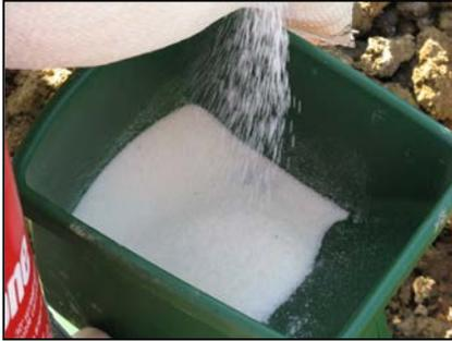
Polyacrylamides (PAMs) are a group of polymers that have been used for decades in a variety of industries. PAMs used for construction site erosion and sediment control (ESC) applications are anionic, high molecular weight, water soluble molecules formed by polymerization of the monomer acrylamide.
