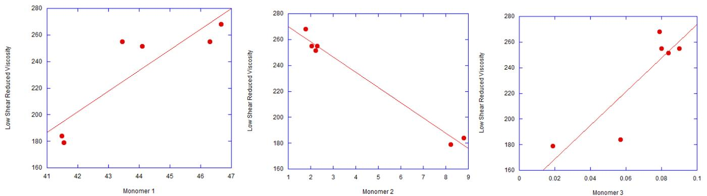
Figure 3: Low Shear Reduced Viscosity vs. Composition for the First of Two Available Grades
