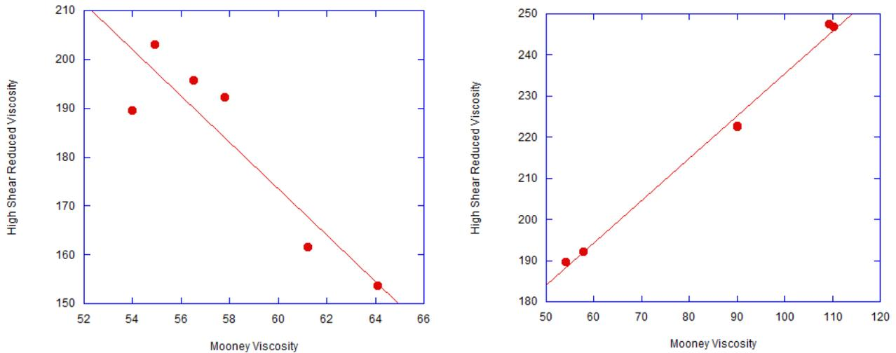
Figure 2: High Shear Reduced Viscosities vs. Mooney Viscosities
