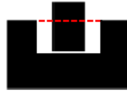
Incorrect Alignment, Front Post too High
