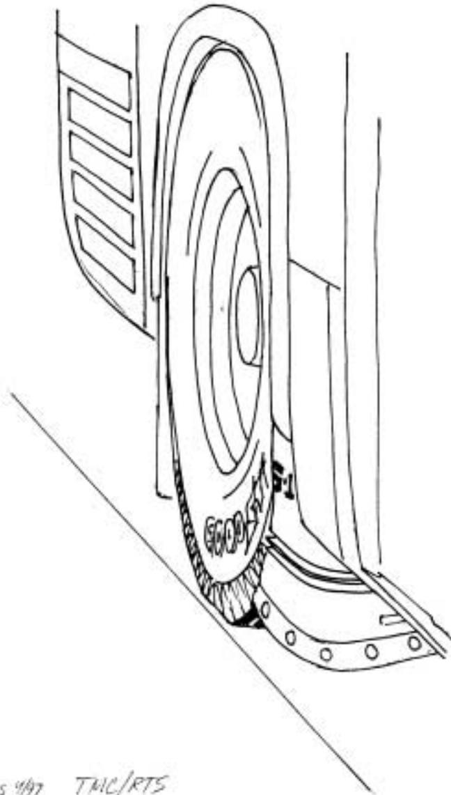
As noted in Figure 2, field trials do support the ability of this design to physically move a subject from the path of travel. This is helpful in instances where Bernoulli's principal is not a causal factor, as when transit buses turn into pedestrians or cyclists. In those instances, the guard must act much like the cowcatcher on a train and physically move the individual from the path of the rotating wheel.
