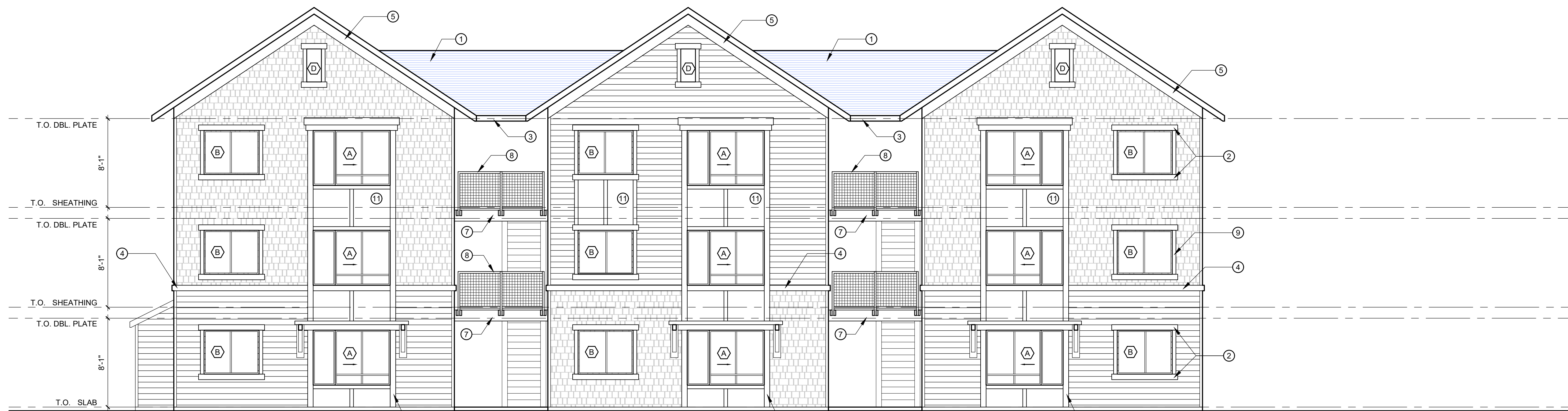
2 BUILDING 100 - WEST ELEVATION A200 3/16" = 1'-0"
