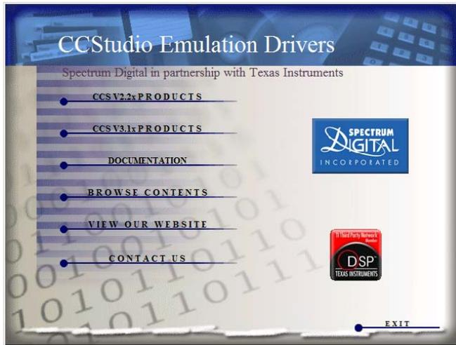
2. Select the CCStudio product version and then the processor of interest. For CCS 2.2x drivers you have the choice of C2000, C6000 and OMAP(C54/C55/ARM). For CCS 3.1x platinum there is only one choice and it includes all processors in one install. When installing emulation drivers the default install should be changed to same directory as you targeted CCStudio install. For CCS 2.2x this is normally "c:\ti" and for CCS 3.1x this is normally "c:\CCStudio\_v3.1".
