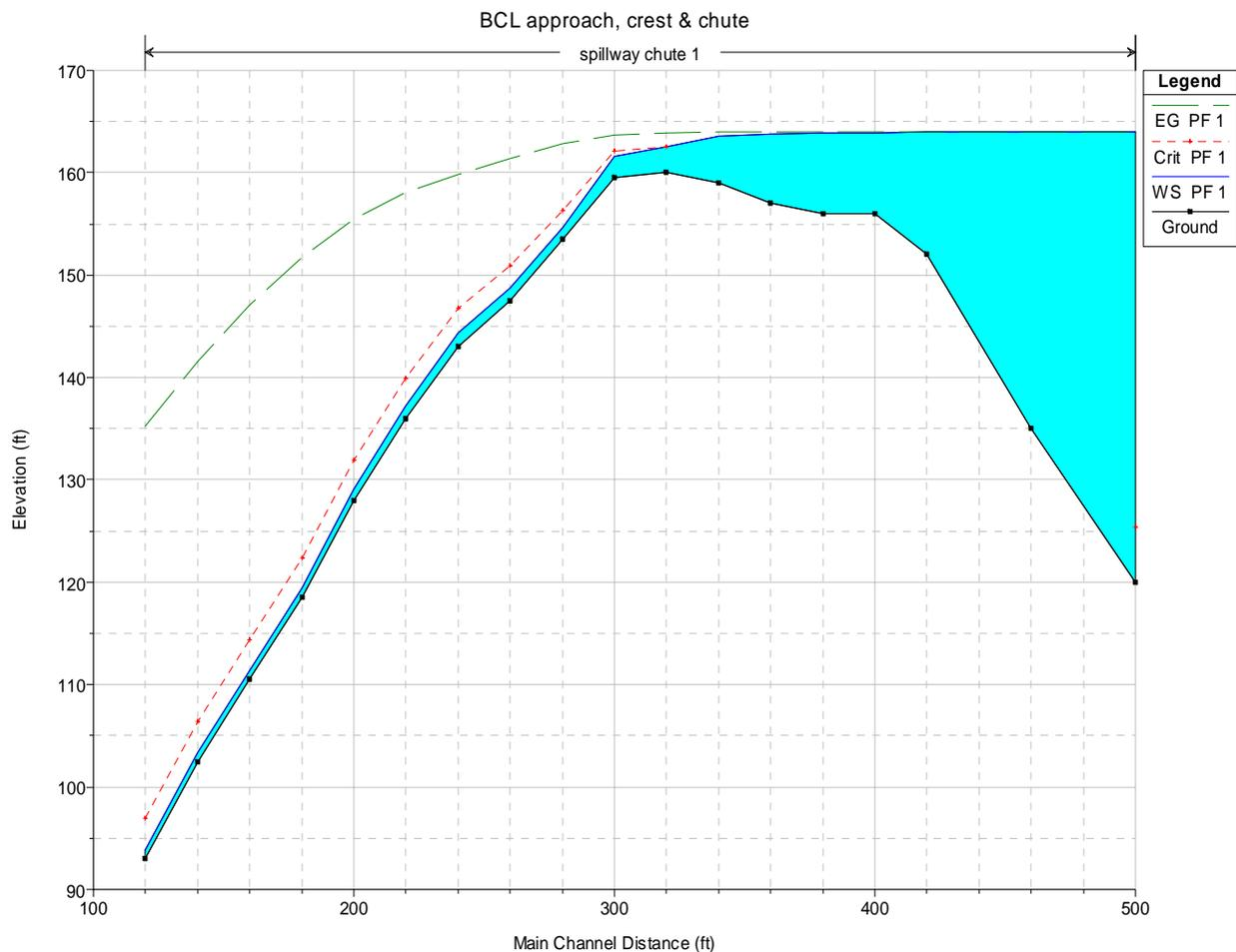
Figure 7. HEC-RAS water surface profile simulation results for steady-state spillway flow of 880 *cfs*. The hydraulic grade line is the water surface. EG is energy grade line, CRIT is water surface profile at critical depth, WS is water surface profile, and GROUND is the elevation along the channel bottom centerline. The spillway crest is at main channel distance of 320 *ft*.
