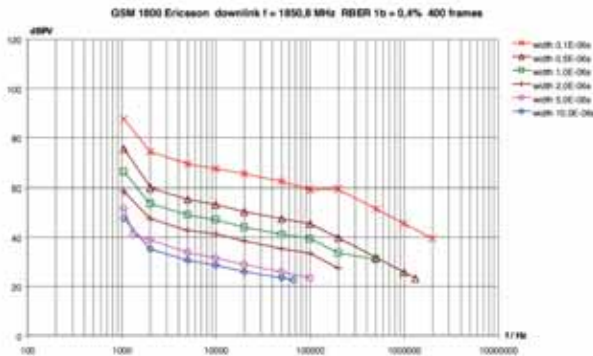
Fig. 1. Effect of impulsive disturbance on GSM radio communication system as investigated in [2].
