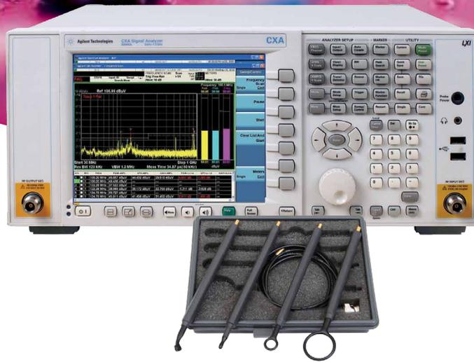
Figure 1 The Agilent N9000A CXA X-Series signal analyzer and N9311X-100 close field probes
