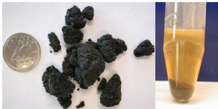
Fig. 6. Oil sands. Left: raw oil sand sample, showing bitumen, water, sand, and clay mixture. Right: Resuspension of oil sands mixture in buffer for DNA extraction from SCODA.
