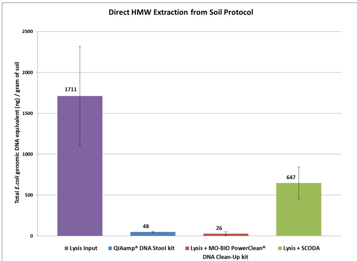
Figure 1. Normalized DNA recovery for each purification method (scaled to account for dilution). Error bars represent standard deviation of PCR replicates (n=2). Data values are calculated according to the following formula: [DNA in PCR]x(volume of protocol output)x(dilution factor)x(sample-size scale factor)
