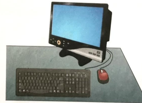
Desktop computer with a CPU inside the monitor
