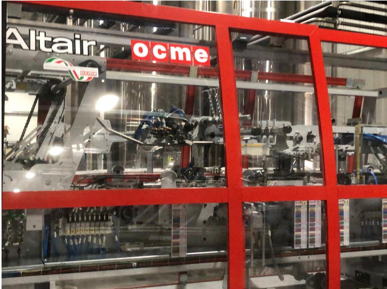
The Ocme tray/case packer handles both four-pack cartons of wine, as well as loose cans in 187- and 375-mL sizes. A bypass lane carries loose 187- or 375-mL cans that will not be packed in cartons to the next piece of equipment on the line: an [Ocme](#) Altair X30 wraparound case/tray packer. Here, the loose cans are either tray-packed or packed in cases holding varying quantities, and four-packs conveyed from the cartoner are placed in trays.
