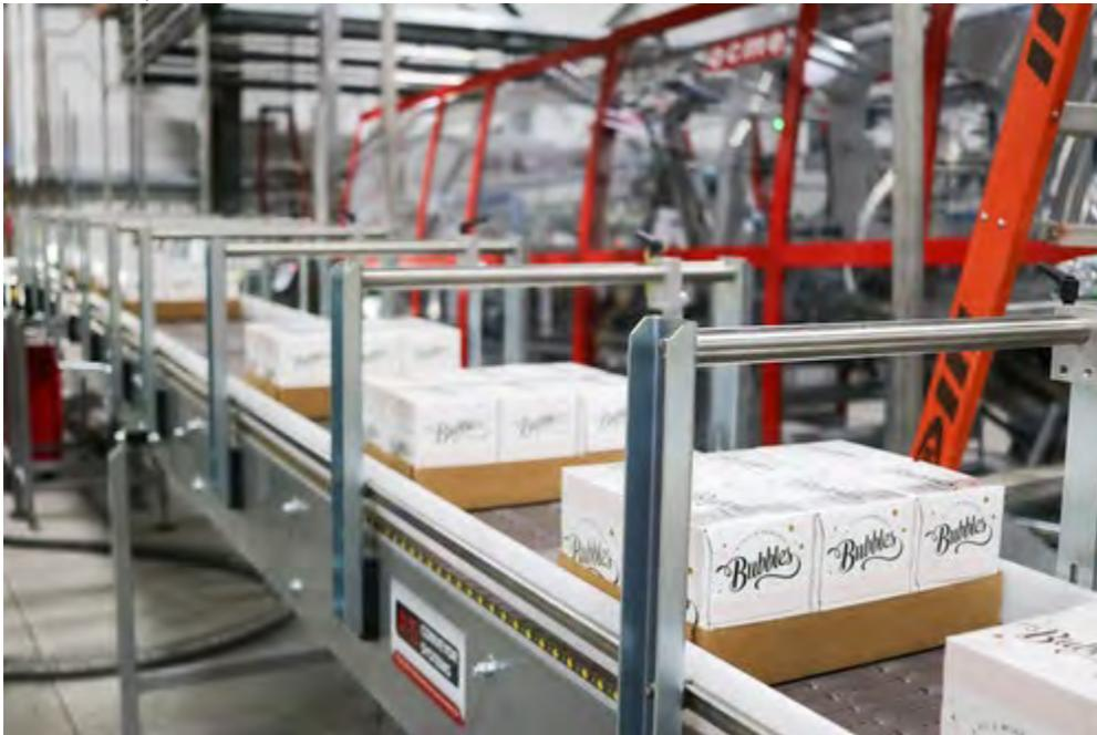
Per TTB regulations, 250-mL cans are packed in four-pack cartons, which are then loaded into trays on the Ocme tray/case packer.
