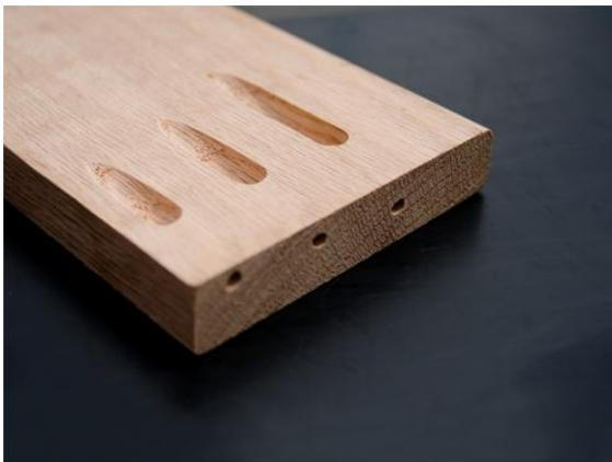
“Unlike others of its kind that use pneumatically driven components, the SPM301 features cam-driven action providing fast smooth cutting action under complete mechanical control throughout the machine cycle,” noted Tom Houska, marketing manager for Safety Speed. “In addition, the SPM301 produces a high-quality 6-degree angle pocket. Higher angles tend to create a high lateral load on the bit, causing bit breakage. Another problem with
