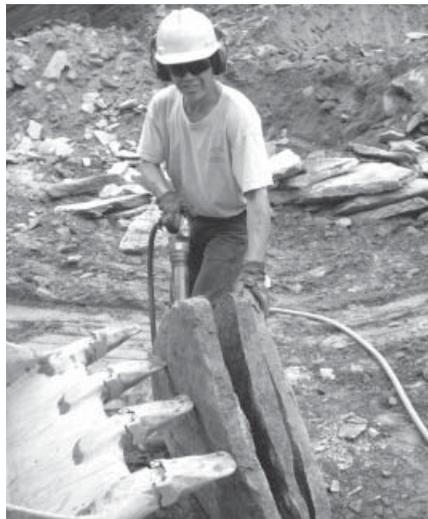
If the excavated stones are thick and large enough and have a naturally square edge they'll be marked for use as steps. Smaller clean edge pieces are wall stone. Wall stone pieces are then sorted for fine and common grade and are dumped into pits. From here dump trucks are loaded and brought back to the yard to
