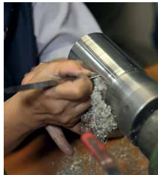
Right Filing and polishing the rough surfaces of newly cast pewter products are done by hand, against a buffing wheel or fine-grade sandpaper. Great skill is required to remove the patina that forms during the casting process.
