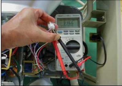
**Picture 2 How to measure voltage**
