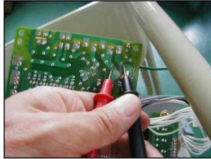
Take out the burner control, and point the lead head at solder part of SA1
