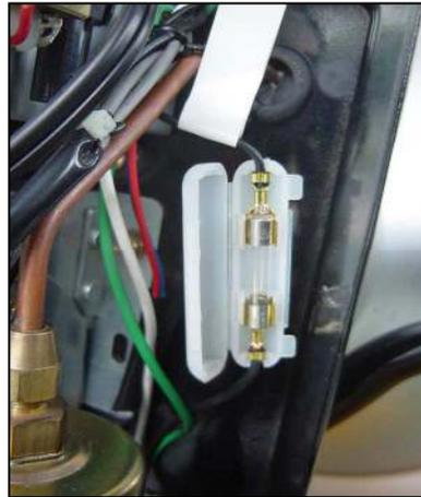
Open the fuse box and check whether the fuse blows out
