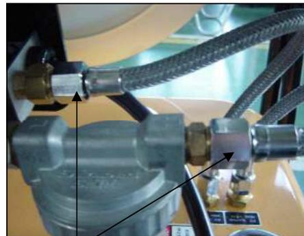
Unscrew two silver nuts with holding gold nuts and remove two fuel hoses
