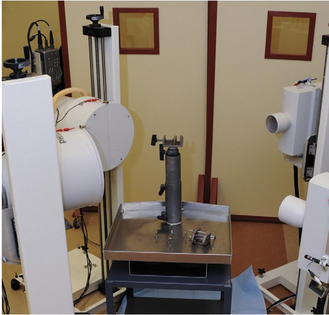
**Fig. 1.** Photo of the biplane fluoroscopy system with the specimen holder positioned as used for the knee extensions. The two fluoroscopy systems were placed at a  $70^\circ$  angle of each other to create the 3D viewing area in which the specimens were imaged.
