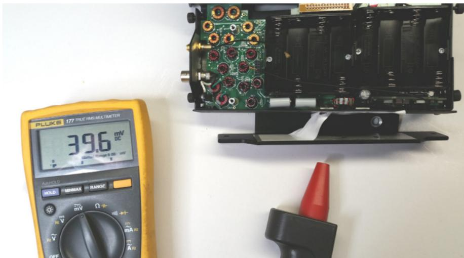
In some cases prying firmly with a flat-bladed screwdriver stuck between the heatsink and one side of the case back may be necessary to initiate separation. When properly performed using a hair dryer, this procedure poses no potential damage to the KX3 or its powder coat finish. Thermal fold-back for the KX3 in normal operation is set by Elecraft at 60°C, and a hair dryer outputs air at about 50-60°C (122-140°F) maximum.
