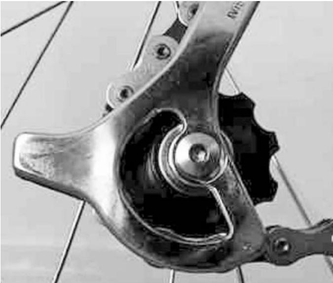
The top cog is very close to the freewheel. When you adjust the gears with the lever on the handlebar, this cog moves sideways to a different gear on the cassette and drags the chain with it. The chain naturally slips from one gear to the next as you turn the pedals.
