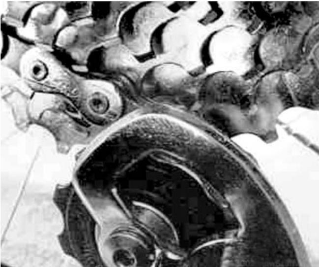
A common mountain bicycle has wheels that are about 26 inches in diameter. The "lowest" gear on the bike might use the tiny "granny gear" front chain wheel with 22 teeth and a rear gear having 30 teeth. That means that the gear ratio is 0.73-to-1. For each turn of the pedals, the rear wheel turns just 0.73 times. In other words, for each pedal stroke, the bike moves forward only about 60 inches (about 5 km/h at a 60-rpm pedaling rate). Like a slow walk. Just what you need to climb a steep hill.
