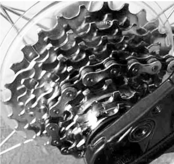
The cassette has between five and ten gears on it, depending on the bike. A freewheel spins freely in one direction and locks in the other. That allows the rider to either pedal or not pedal -- when not pedaling, the bike **coasts** (another feature that tricycles and penny-farthing bicycles lack).
