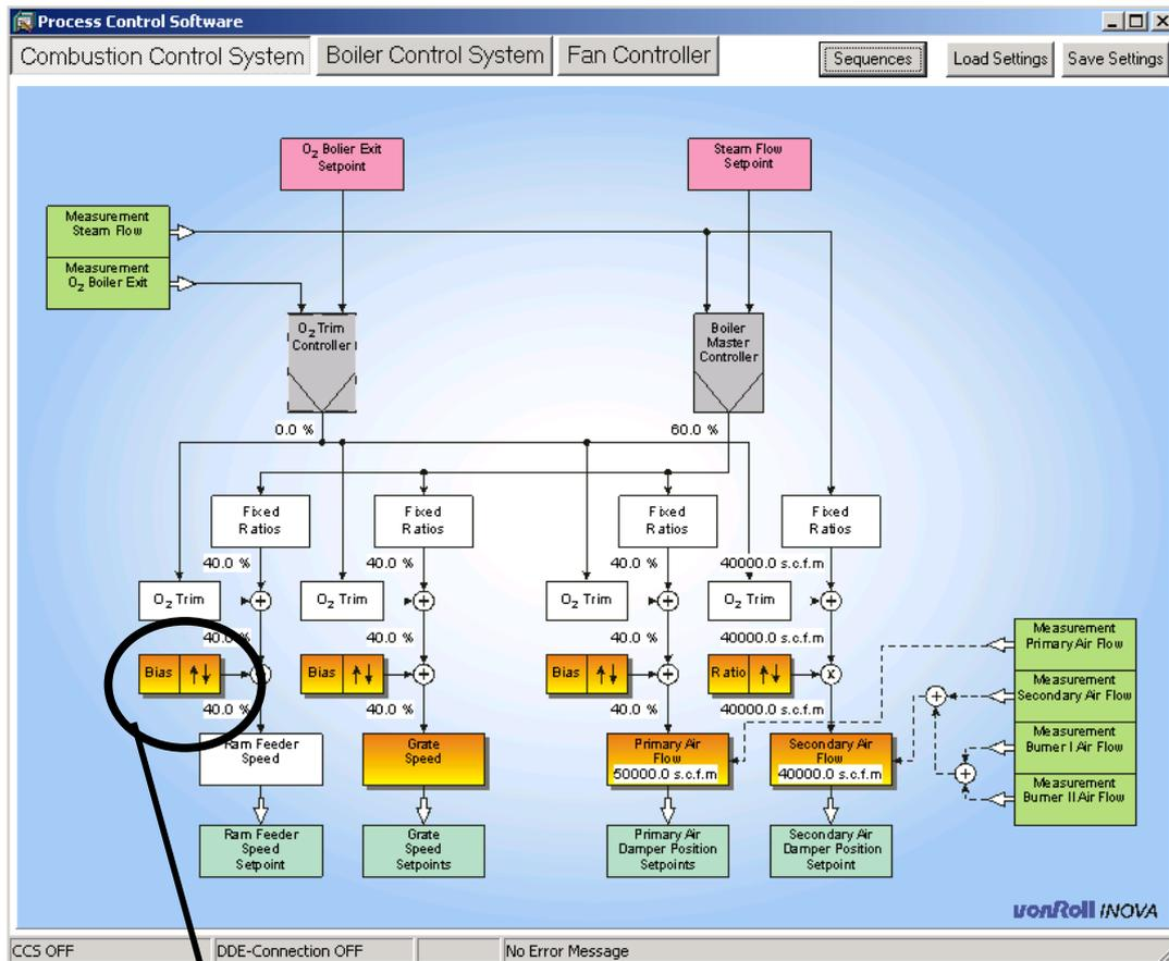
Fig. 4 & 5 Combustion Control Screen and bias controls
