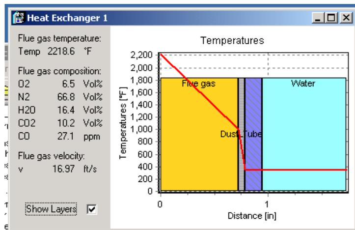
Figure 7: Flue gas detail at boiler tube
