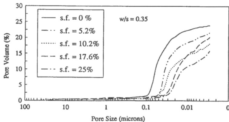
Figure 5 Pore size distribution in the cement-silica fume composite system.
