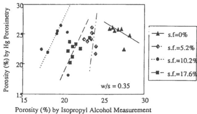
Figure 4. Porosity of cement composite systems containing various amount of silica fume and wollastonite micro-fibres. Values determined by Hg intrusion porosimetry versus values determined by isopropyl alcohol saturation.
