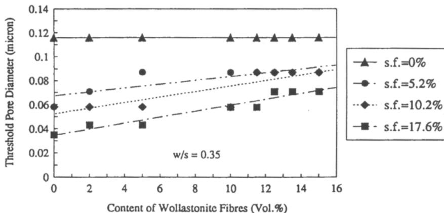
Figure 10. Threshold pore diameters of cement-wollastonite and cement-silica fume-wollastonite composite systems containing different amount of silica fume in mixtures.
