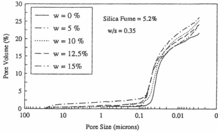
Figure 7. Pore size distribution in the cement-silica fume-wollastonite composite mixtures containing 5.2% silica fume.
