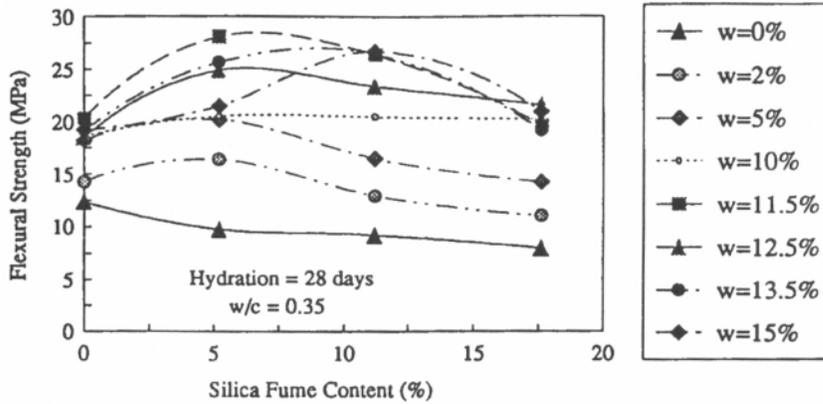
Figure 1. Variation of flexural strength with silica fume contents for cement composite systems containing different amount of wollastonite micro-fibres in the base matrix.
