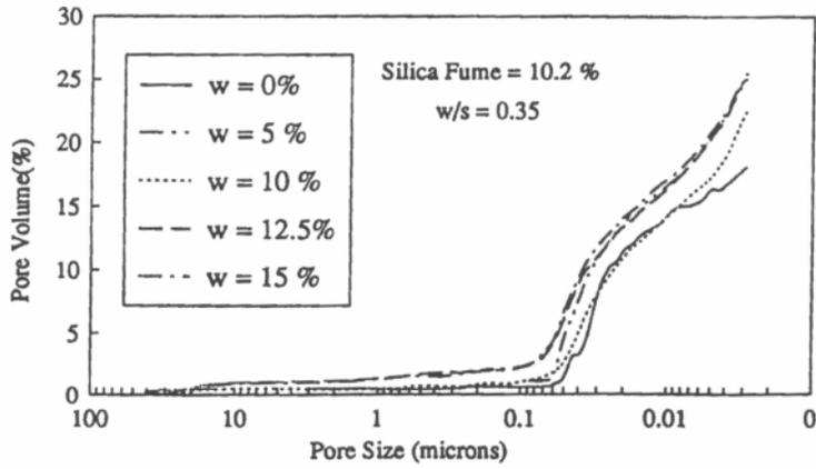
Figure 8. Pore size distribution in the cement-silica fume-wollastonite composite mixtures containing 10.2% silica fume.
