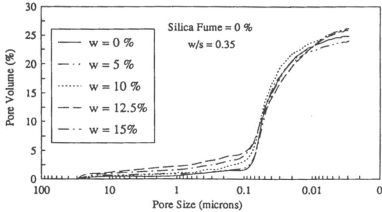
Figure 6. Pore size distribution in the cement-wollastonite composite system.
