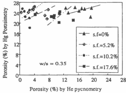
Figure 3. Porosity of cement composite systems containing various amount of silica fume and wollastonite micro-fibres. Values determined by Hg intrusion porosimetry versus values determined by He gas pycnometry are plotted.
