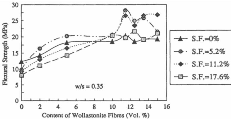
Figure 2. Variation of flexural strength with concentration of wollastonite micro-fibres for cement composite systems containing different amount of silica fume in the base matrix.
