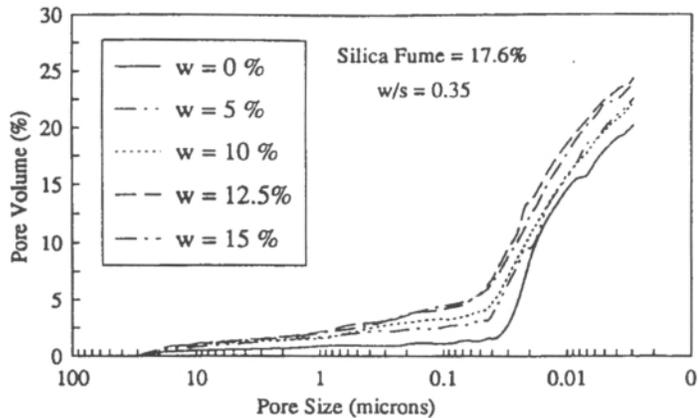
Figure 9. Pore size distribution in the cement-silica fume-wollastonite composite mixtures containing 17.6% silica fume.
