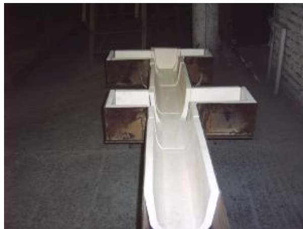
Fig. 7 Sections of cast spouts for aluminum transition lines
