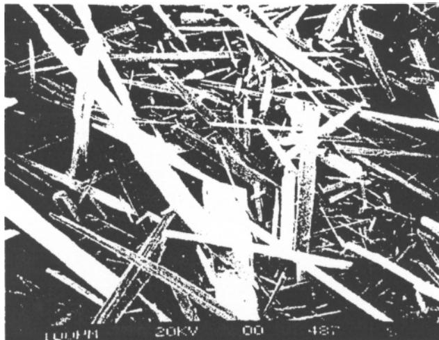
Figure 1. SEM micrograph of the natural wollastonite micro-fibres.
