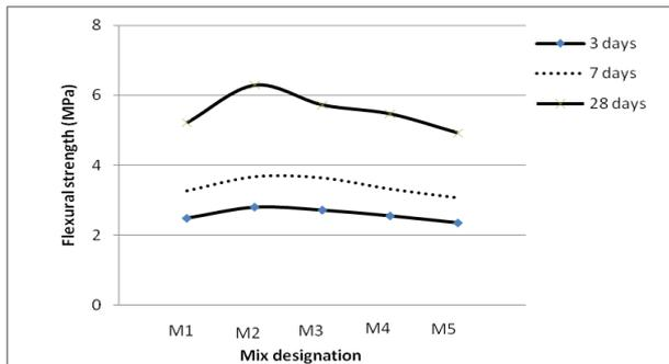
Fig.2. Flexural strength of hardened concrete with or without WMF.
