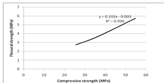
Fig.6. Correlation between flexural and compressive strength of M3
