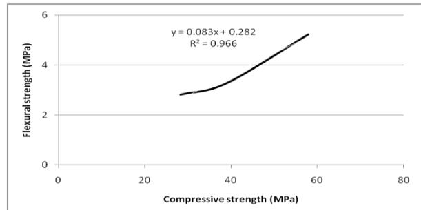
Fig.4. Correlation between flexural and compressive strength of M1
