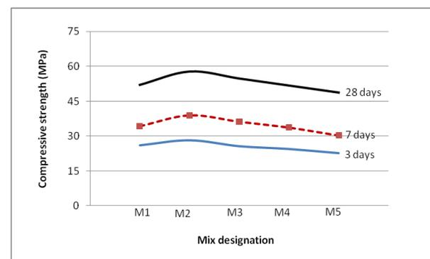
Fig.1.Compressive strength of hardened concrete with or without WMF.
