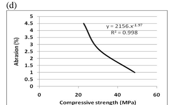
Fig. 10. Best fit between abrasion and compressive strength (a) M1; (b) M2; (c) M3; (d) M4 and (e) M5.
