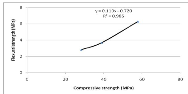
Fig.5. Correlation between flexural and compressive strength of M2
