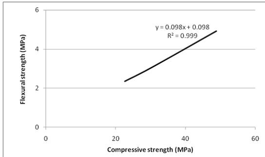
Fig.8. Correlation between flexural and compressive strength M5
