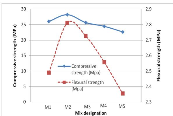
Fig.3. Compressive and flexural strength of concrete with or without WMF.
