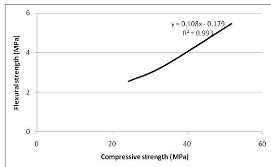
Fig.7. Correlation between flexural and compressive strength of M4
