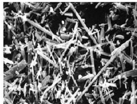
Fig.2. SEM image of Wollastonite micro-fiber.
