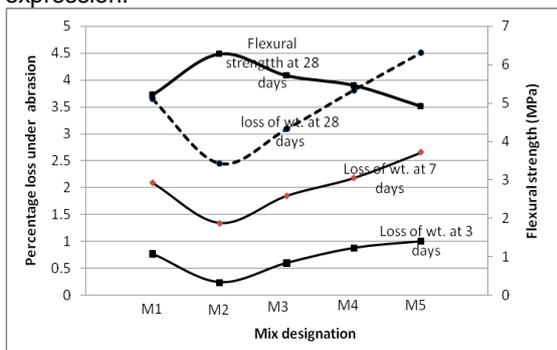
Fig. 9. Correlation between flexural strength at 28 days and % loss of weight under abrasion
