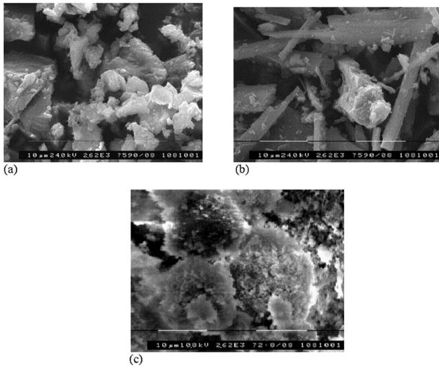
**Fig. 1.** SEM of materials (a) OPC; (b) wollastonite; and (c) microsilica
