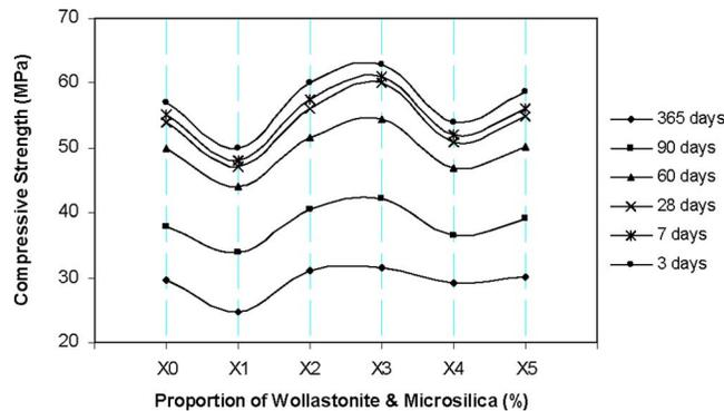
**Fig. 10.** Relationship between compressive strength of OPC-wollastonite-microsilica mortar and proportion of wollastonite and microsilica in mix
