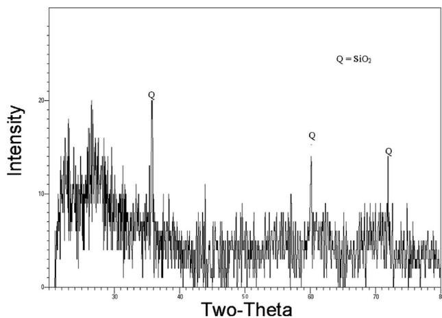
**Fig. 4.** XRD pattern of 100% microsilica paste after 28 days of curing
