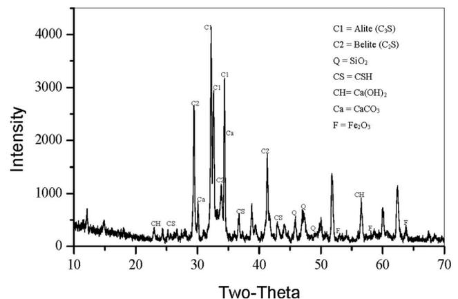
**Fig. 2.** XRD pattern of 100% OPC paste after 28 days of curing
