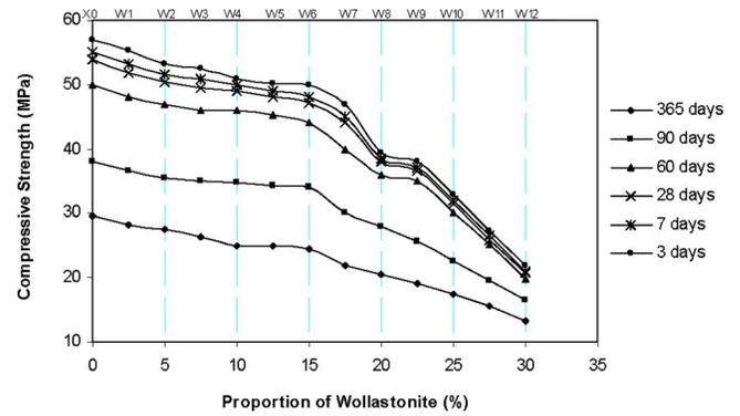
**Fig. 8.** Relationship between compressive strength of OPC-wollastonite mortar and proportion of wollastonite in mix
