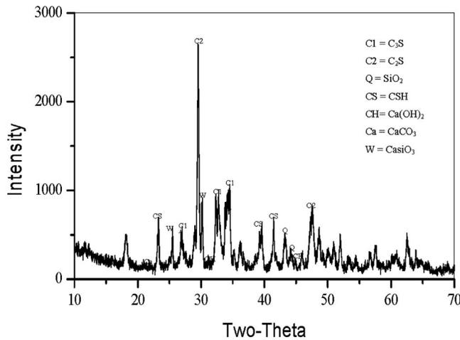
**Fig. 7.** XRD pattern of OPC: wollastonite: microsilica paste in the proportion of 82.5:10:7.5 after 28 days of curing
