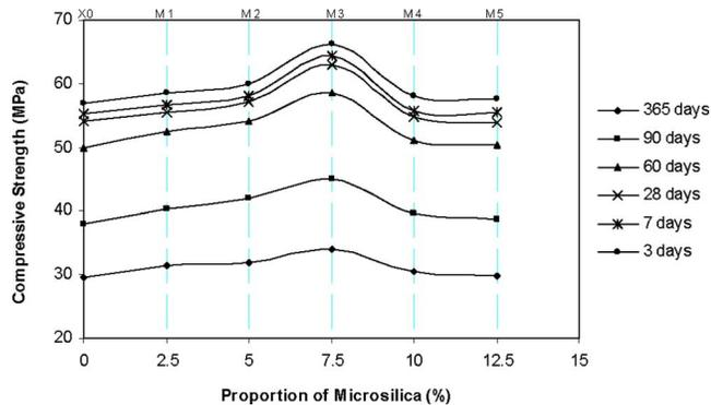
**Fig. 9.** Relationship between compressive strength of OPC-microsilica mortar and proportion of microsilica in mix
