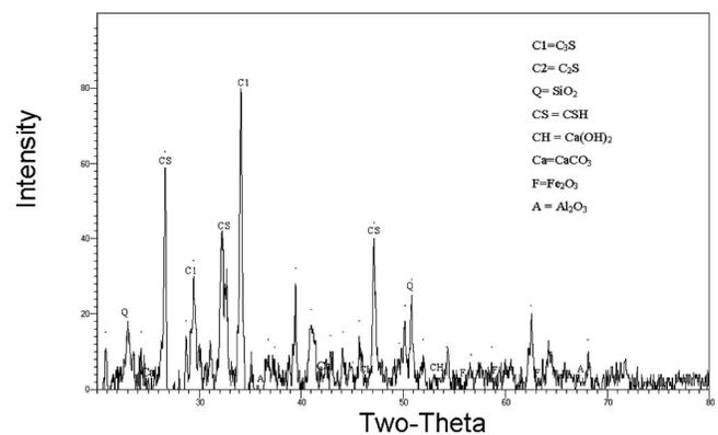
**Fig. 6.** XRD pattern of OPC: microsilica paste in the proportion of 92.5:7.5 after 28 days of curing
