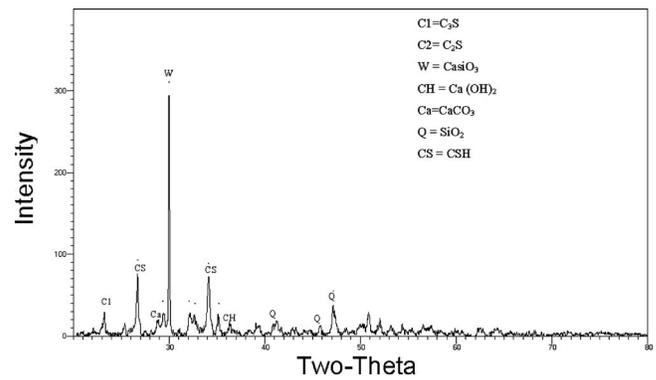
**Fig. 5.** XRD pattern of OPC: wollastonite paste in the proportion of 85:15 after 28 days of curing
