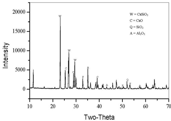
**Fig. 3.** XRD pattern of 100% wollastonite paste after 28 days of curing
