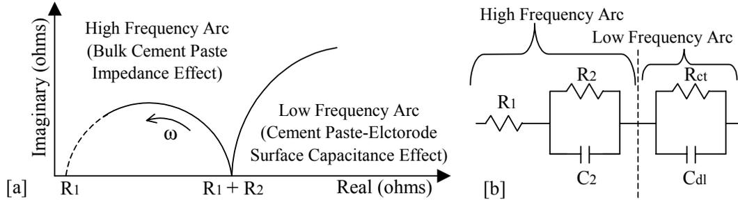
Figure 1 [a] Schematic plot of a high frequency arc in the impedance complex plane obtained for cement paste systems [b] A simplified electrical equivalent circuit for hydrating system.  $R_1$ ,  $R_2$  and  $C_2$  are high frequency resistance, solid-liquid interface resistance and capacitance.  $R_{ct}$  and  $C_{dl}$  are cement-electrode interface charge transfer resistance and double layer capacitance.
