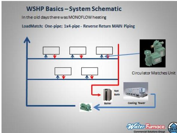
Note the difference above. The mains remained the same as reverse-return and can be horizontal or vertical mains. The One-Pipe distribution pipe (LOOP) is sized like a coil for the load served. The pipe is sized at a design Delta-T. The result is that the units will all heat
