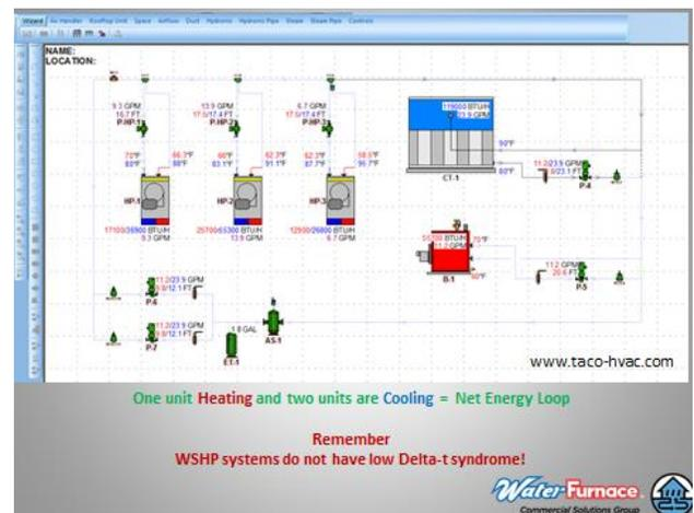
The One-pipe GeoExchange System has been applied repeatedly in Schools where the ground loop is parallel piped to 1x4-pipe WSHP’s.
