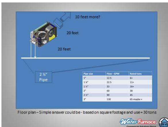
The limitation is the size of pipe selected and the equated tonnage as sized to the load served; not the equipment. This points to a
