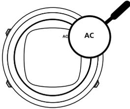
The **AC** is shown until the water contact deactivates. It is important to keep the water contact area clean. Contamination or dirt can prevent automatic activation/deactivation.
