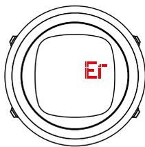
If you omit decompression stops for longer than three (3) minutes, the RGBM algorithm is locked for 48 hours. When the algorithm is locked, no algorithm information is available and **ER** is shown instead. Locking the algorithm is a safety feature, highlighting that the algorithm information is no longer valid.
