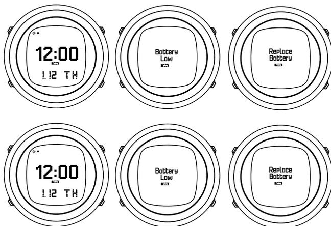
If the low battery icon appears in surface mode, or if the display looks faded, the battery may be too low. Battery replacement is recommended.
