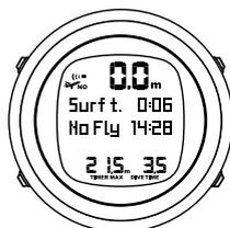
No-fly time is always at least 12 hours and equals desaturation time when it is more than 12 hours. For desaturation times shorter than 70 minutes, the no-fly time is not displayed.
