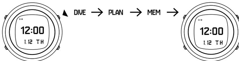
Time and dive modes have different views in the bottom row which you can scroll through with [DOWN] and [UP].
