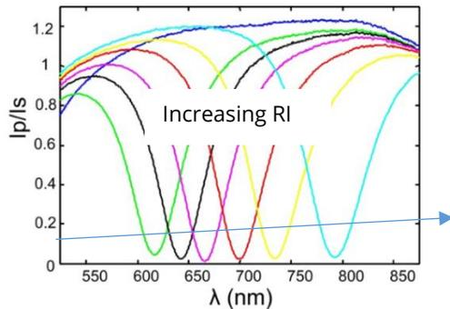
Figure 3 – Reflectance spectra (light polarisation ratio) of solutions with different RI on an Au SPR sensor in wavelength interrogation mode.
