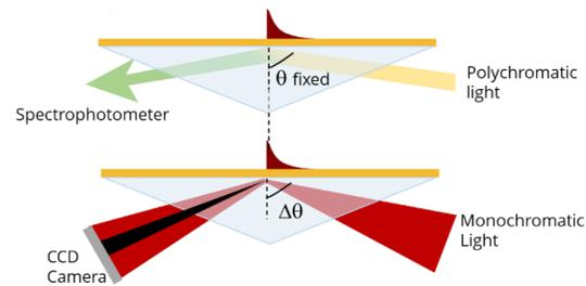
Figure 4 - Wavelength (a) and angular (b) interrogation.
