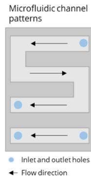
Figure 8 - P4SPR microfluidic cell design.
