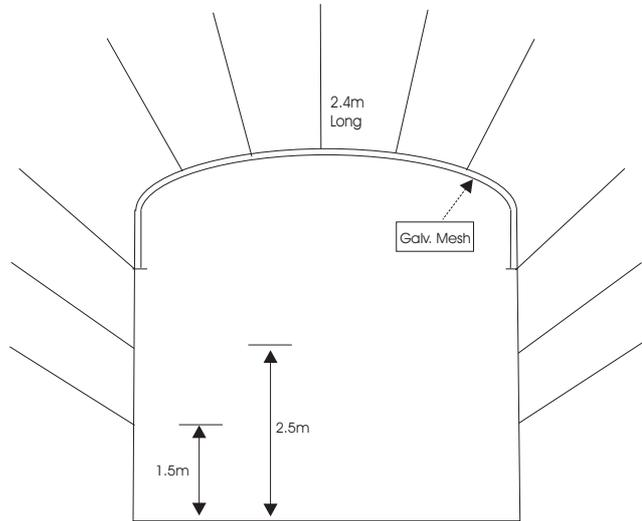
FIG 5 - Standard rockbolting and meshing pattern (section view).
