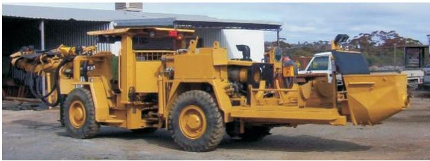
FIG 7 - Lightning Nickel shotcrete. Atlas Copco 282 carrier.
