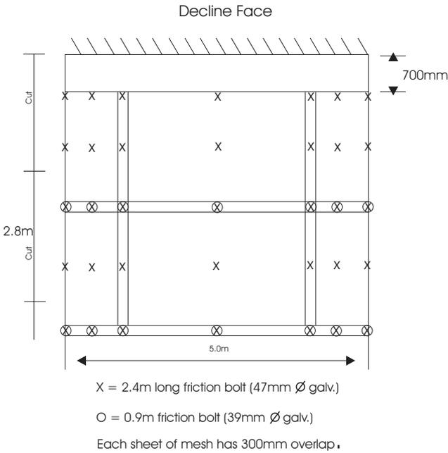
FIG 4 - Standard rockbolting and meshing pattern (plan view).
