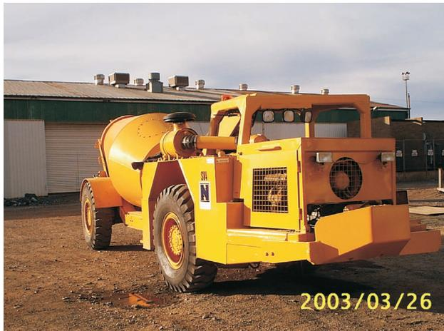
FIG 8 - Lightning Nickel agitator, Normet NT120 carrier.
