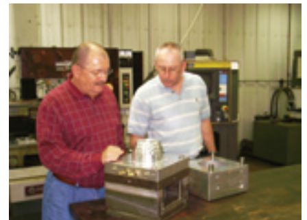
Gordon Tubbs (left), tooling designer and Scott Cain (right), programmer, look over the core and cavity after machining.
