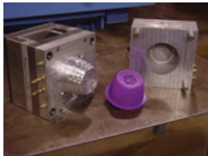
This core and cavity was machined on a Mazak V65/60 vertical milling machine at 1,500 rpm, 12 ipm using a ½-inch HS cutter.
