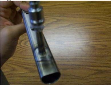
**Figure 3 Brazed Fuel Distribution Manifold**
