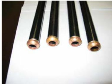
**Figure 7 Brass Ferrule to Stainless Tube**
