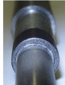
**Figure 20 Hydrogen Quartz Tube Nickel Brazed 2250° F**
