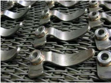
Lever Photograph of Copper Braze Ring pre-placed in Position for Furnace Brazing
