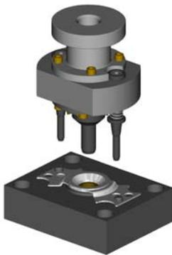
Illustration: Press Assembly Tool to Facilitate a "Press-Fit"
