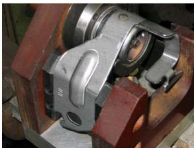
**Figure 5 Airbag Component: Photograph of Spot Weld Fixture Required to Hold Parts In Position for Furnace Brazing**
