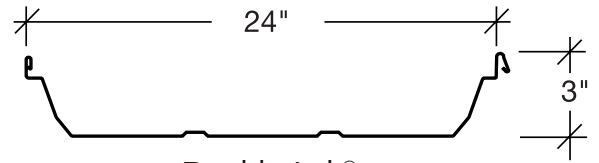
Double-Lok® Field Seamed System 12" and 18" also available
