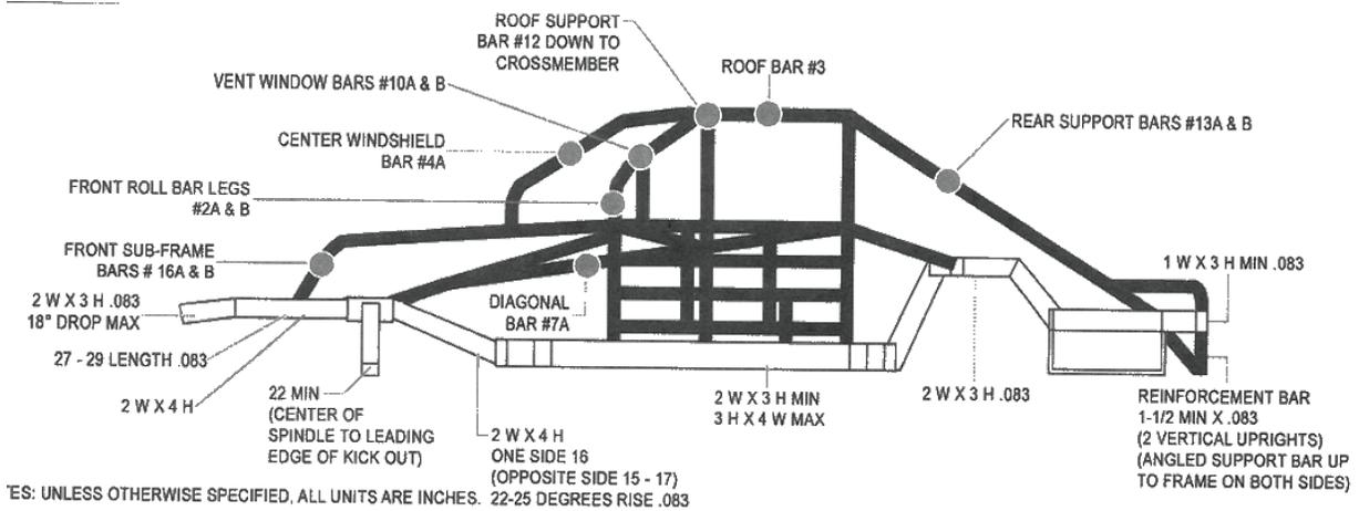
DIAGRAM 4 - EXPLODED VIEW OF BASIC ROLL CAGE
