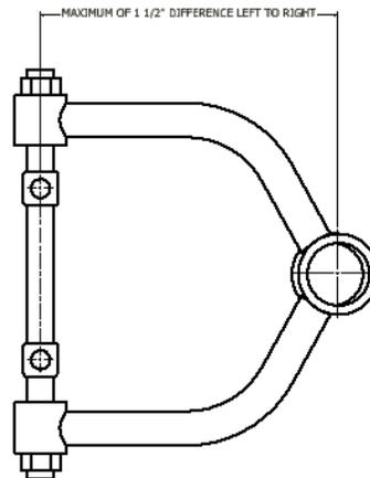
12. The maximum shim stack on the upper A-frame is ½ inch, this will include solid bars and shims
