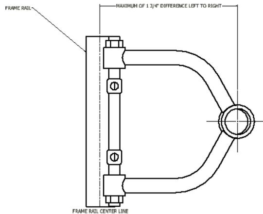
11. The upper A-frames must be within 1 ½ inch of each other, when measured from the center of the bushing hole to the center of the ball joint. See diagram below:
