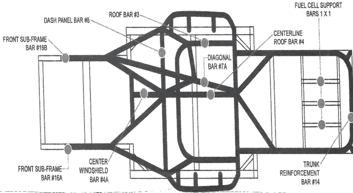
DIAGRAM 3 - TYPICAL ROLL CAGE AND FRAME CONSTRUCTION (SIDE VIEW)
