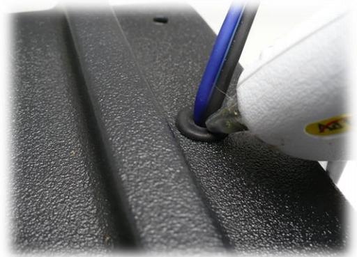
Use a glue gun (or similar medium) to plug any remaining air space around speaker wires as they exit the grommet to ensure an air-tight seal (air escaping could make a whistling noise on bass notes).
