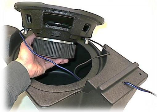
Install rubber grommet in underside hole and run speaker wires through to connect to your subwoofer. Place sub in pod and gently pull any excess speaker wire back through the grommet. This may take a few attempts... you want it slightly loose but excess wire could vibrate if it's touching the pod walls.
