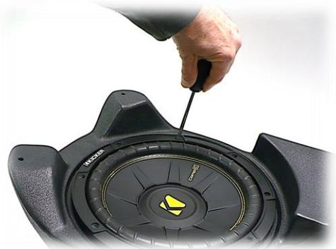
...but it's a good idea to **finish** tightening by hand to avoid stripping the plastic in case you have a pretty powerful drill. ☺
