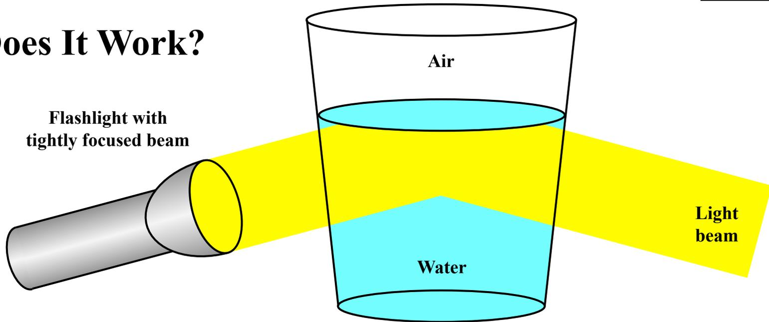
Fiber optics work because of total internal reflection. When light traveling through water bounces at a shallow angle off the surface between water and air, the light prefers to stay in the water, where it can travel more slowly. However, if the light beam angles upward more, it will escape to the air, not bounce back into the water.
