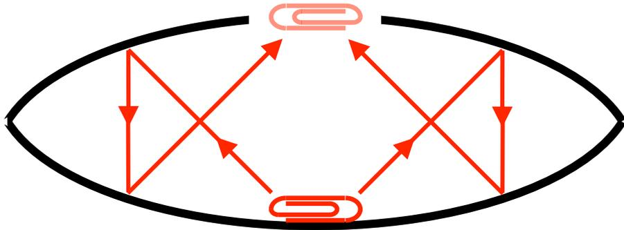
Light from an object at the bottom of the mirage maker bounces off the curved mirrors to create an image of the object at the top of the mirage maker
