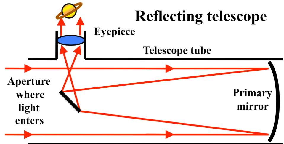
Curved mirrors can be used (just as lenses can be) to create magnified images in telescopes and microscopes. Large mirrors are cheaper and lighter than large lenses.
