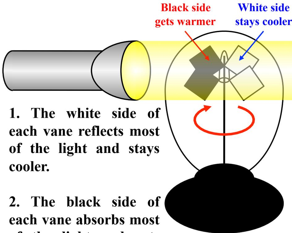
1. The white side of each vane reflects most of the light and stays cooler.
