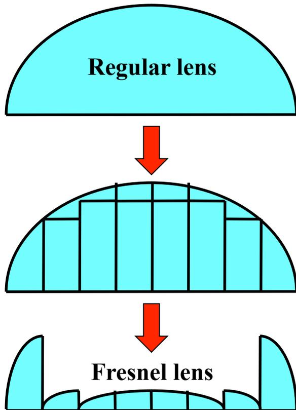
A Fresnel lens (with concentric circles) is flatter and lighter than a regular convex or concave lens.
