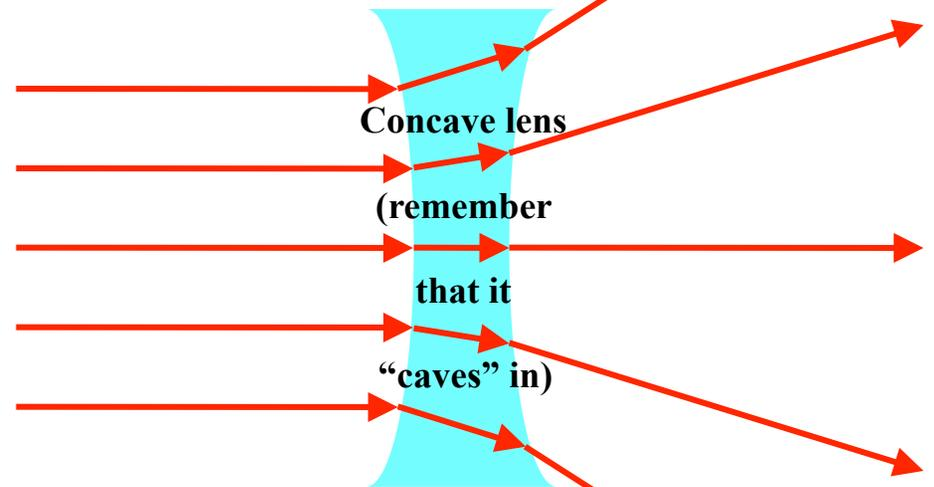
Shaped glass or plastic lenses bend light rays in desired directions
