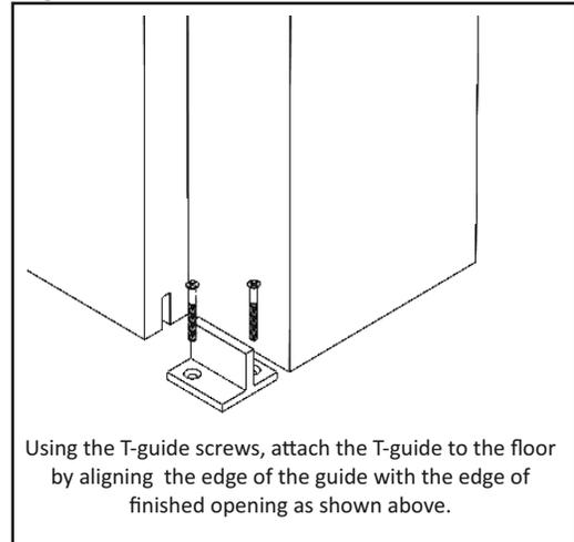
Using the T-guide screws, attach the T-guide to the floor by aligning the edge of the guide with the edge of finished opening as shown above.
