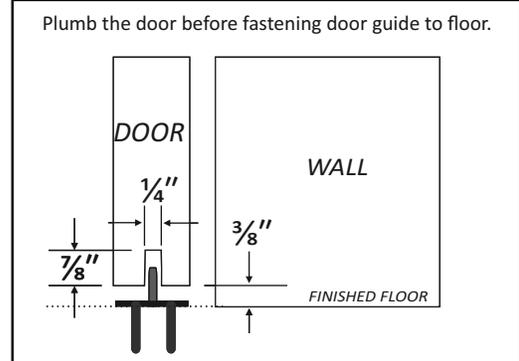
Plumb the door before fastening door guide to floor.
