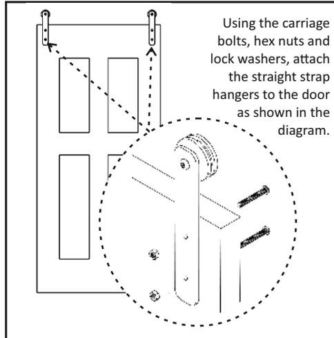
Using the carriage bolts, hex nuts and lock washers, attach the straight strap hangers to the door as shown in the diagram.
