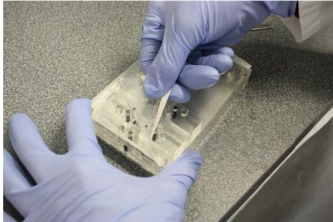
Figure 2. Removing the sealing film from the cartridge.
