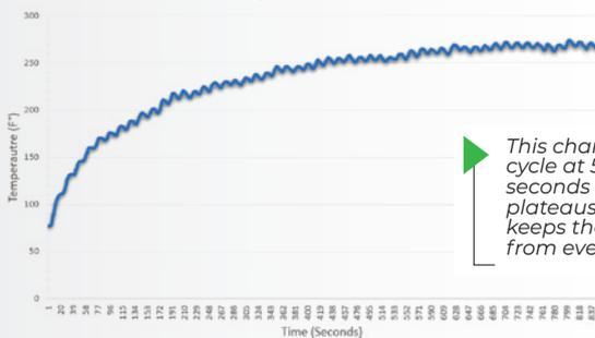
This chart shows a 33% duty cycle at 5 seconds on and 10 seconds off. The DHT-400 plateaus at ~270°F which keeps the sensitive elements from ever reaching 400°F.
