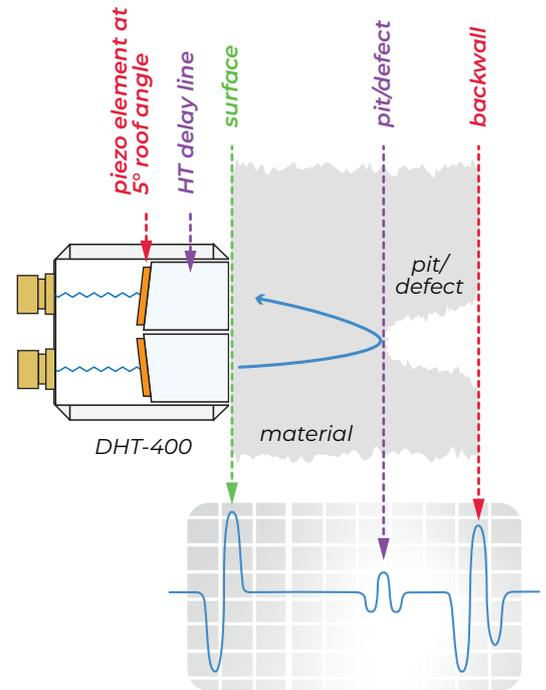
The two 5° roof angles create a pseudo-focusing effect thereby increasing the transducer's sensitivity for pit-like defects.
