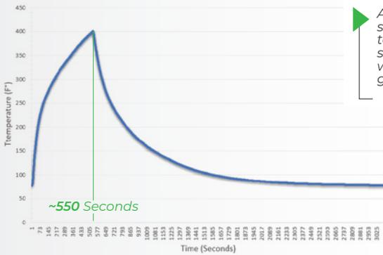
At 932°F continuous surface contact temp, it takes over 9 minutes for the sensitive solder joints within the transducer to get to a 400°F.
