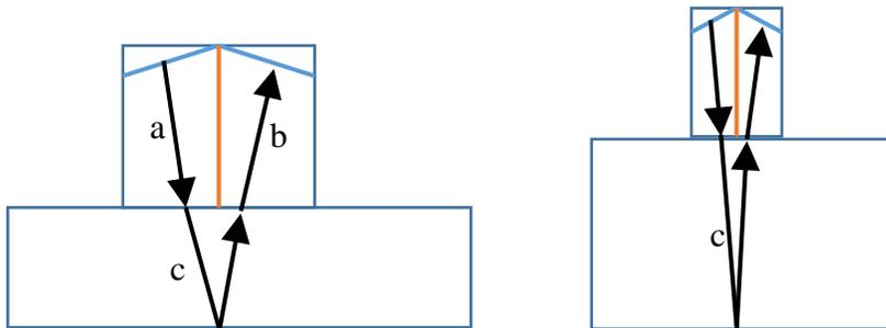
**Figure 5: Dual element delay line concept**
