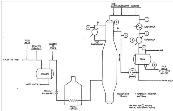
**Figure 8: Schematic view of refining crude unit showing corrosion monitoring locations.**
