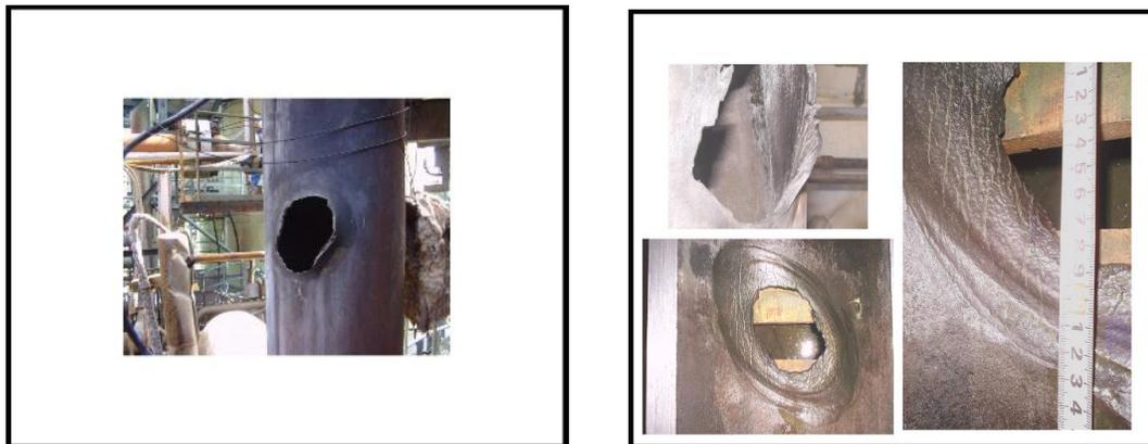
**Figure 9: Pipe failures due to Injection/Mix-point corrosion.**
