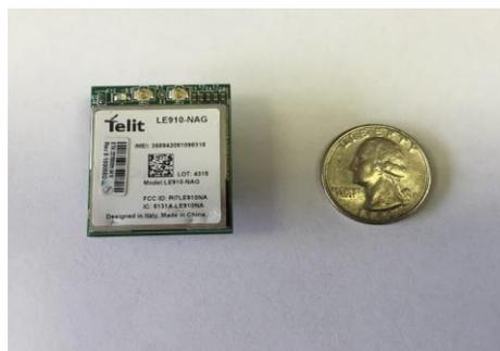
Figure 6: Embedded Modem size comparison
