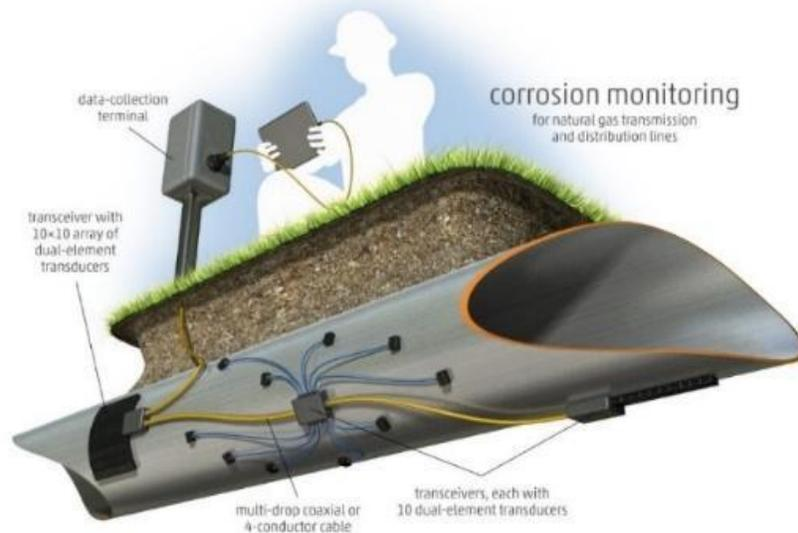
Figure 2: Installed sensor corrosion monitoring application for buried pipelines.
