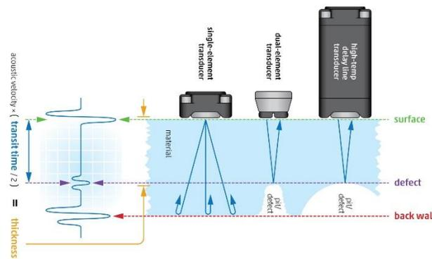
**Figure 1: Ultrasonic Testing principle measures the round-trip transit time of the acoustic energy in the material under test. Wall thickness is calculated from the time measurement.**
