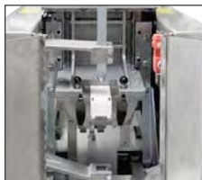
Standard measuring piston replaced by Mini Piston 35-250 g
