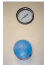
Stepless adjustable pneumatic system for very gentle handling of different types of dough
