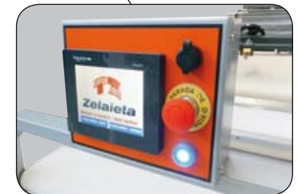
Control panel by automat
