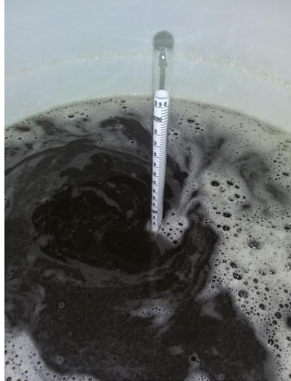
A hydrometer measures the specific gravity (relative density) of a liquid. As yeast converts honey syrup into alcohol, the density decreases.
