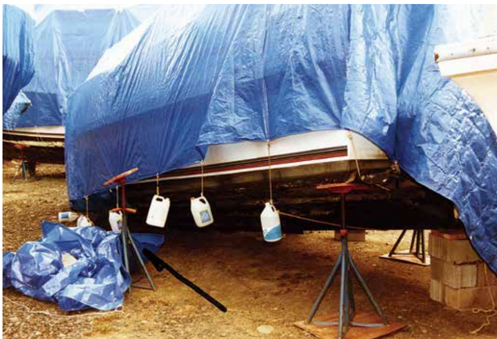
A boat stored ashore needs to be properly supported to make it through winter unscathed.
