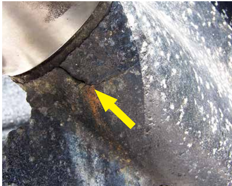
Store outdrives and outboards in the down position so water can drain; otherwise ice can crack the housing.
