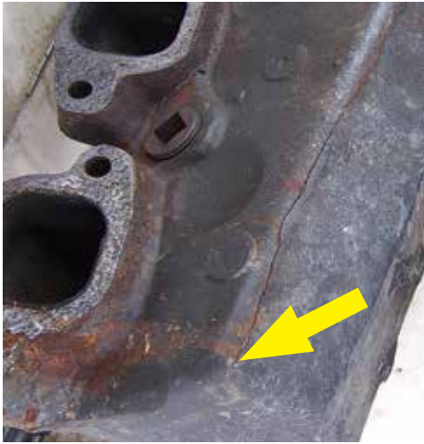
Even a short freeze can cause expanding ice to crack a manifold.
