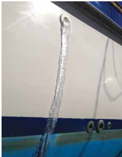
Frozen meltwater can damage thru-hull fittings.
