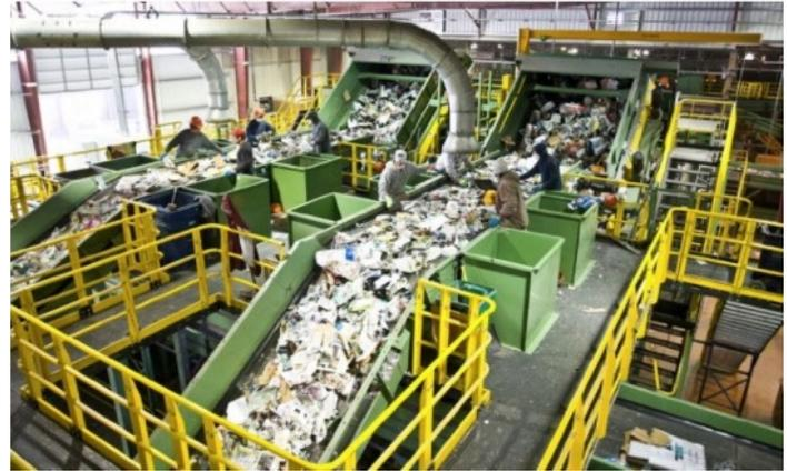
After sorting, various types of waste are conveyed to a specific place by conveyor. For example, ferrous metals go into a large hopper, which is recycled when filled. Food waste is sent to a bioreactor where it produces compressed gas.
