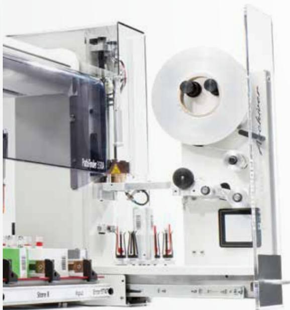
Easy access to load new capping foil
