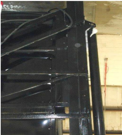
2) Each pivot point has a grease zerk
