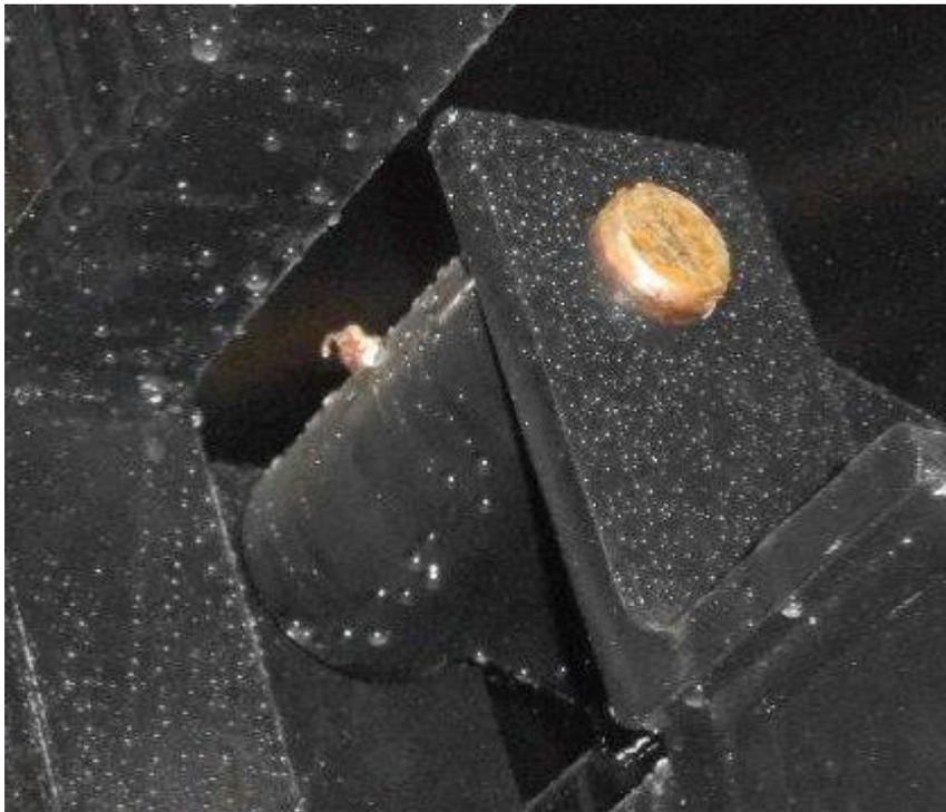
3) Each cylinder has 1 zerk on each end
