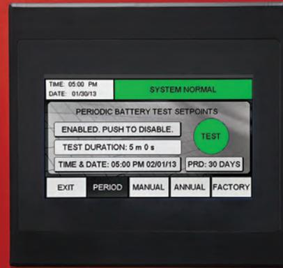
The color touchscreen display on the **Intellistat TS** provides all electrical parameters, inverter status, programmable inverter and battery testing, and data-logging. Optional **NetMinder™** communications allow for remote monitoring and reporting via **BACnet/IP** or **BACnet MS/TP**, **Ethernet TCP/IP**, **MODBUS TCP**, or **MODBUS RS485**. For more details, see the **Remote Communications** description on Page 7.
